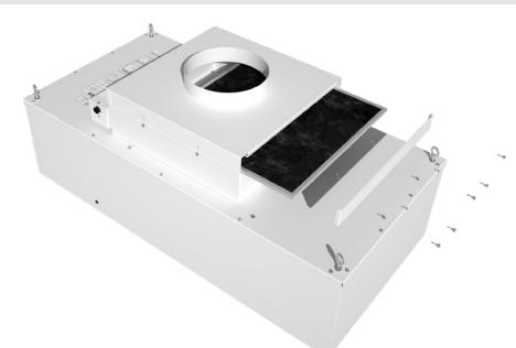
**Step 3:** Clean pre-filter by hand washing in water with a mild detergent or by using a vacuum cleaner. Allow pre-filter to dry completely before replacing.
