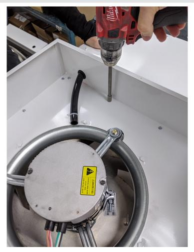
Step 6: Remove motor/blower assembly from the inlet collar by removing the 6 lock-nuts using a deep 7/16" socket wrench (or equivalent).
