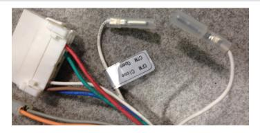
Switching from constant torque to constant flow: To switch the motor from constant torque to constant flow all that is required is to close the connection of the white wire as shown.
