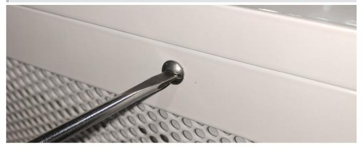
Step 2: Remove filter by loosening cam latch bolts (filter retainer clips) by turning counter clockwise using your hands, or hex key as required to fully tighten latches.
