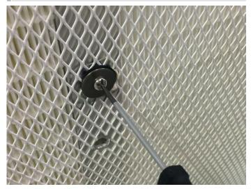
Step 3: Remove threaded standoff and lock washer from LED cable assembly.
