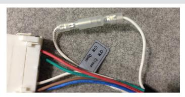
The motor will be factory wired to the motor program selected on the order.
